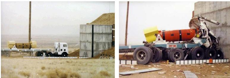
**Test of the durability of containers for spent nuclear fuel**
