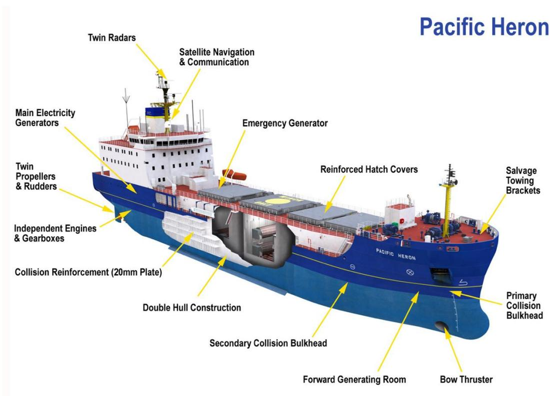
Schematic of 5,000 Tonne Nuclear Material Shipping Vessel
